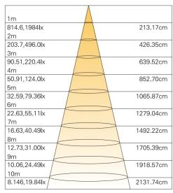
Height Eavg, Emax Angle: 96deg Diameter
